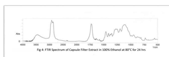
The Spectrum of extracts from *AseptiCap KS* capsule filters with 100% ethanol under extreme extraction conditions show presence of various components used in the manufacture of **mdi** PES membrane capsule filters.
